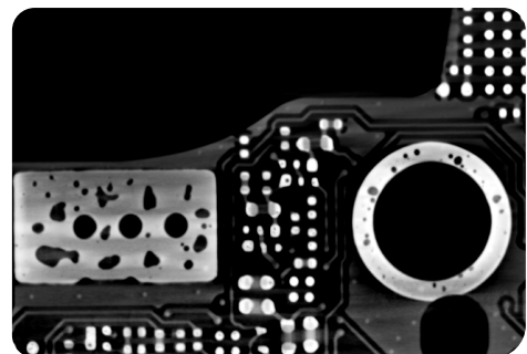
SMT inspection: BGA/QFN evaluation with CT confirmation
